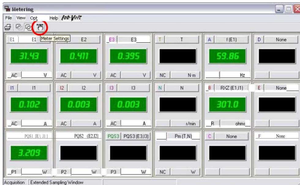
To do this, go to the Meter settings interface and select the appropriate meter, type, and input/function.
