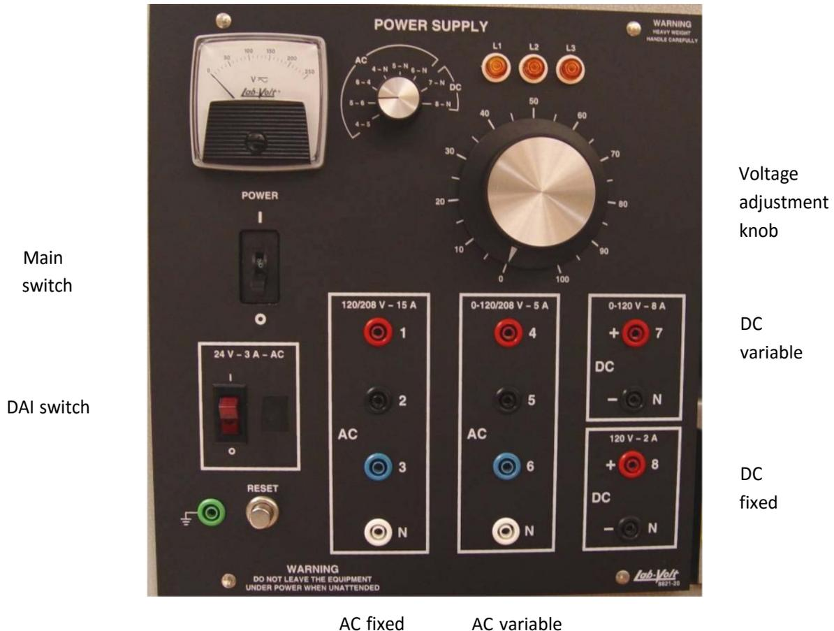
The power supply module has five outputs:
