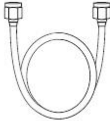
Figure 6: SMA (m) to SMA (m) Cable
