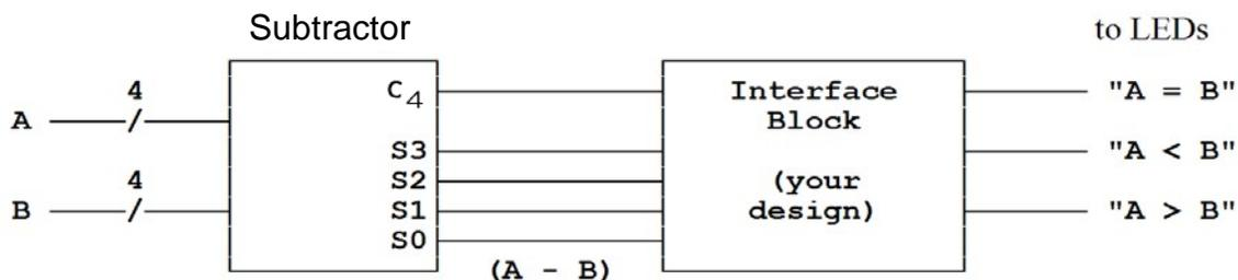
Design the contents of this interface. You will build the circuit using only 2 chips:
