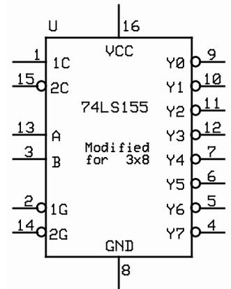
At the right is a 2x4 decoder, a smaller version of the 74155 showing the connections inside. The diagram was obtained online and the labels used are different from the 74155. In the 74155, C is the msb (most significant bit) so X connects to C. In the 2x4 diagram, A is the msb so X connects to A (not B). Otherwise, the basic construction is the same.
