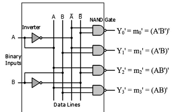
As you can see, the decoder outputs all possible minterms (complemented). So by including a decoder in your circuit, you don't have to use gates to *create* the minterms that you want (as in Exp 6), you only have to *select* them at the decoder output and then collect them together with an external OR gate, or an invert-OR in this case.
