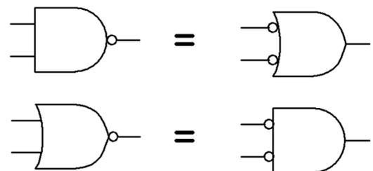
If we think in terms of logic gates, then case (i) means that a NAND gate can be an AND-INVERT (an AND gate with an inverted (bubbled) *output*) or an INVERT-OR (an OR gate with inverted (bubbled) *inputs*).
