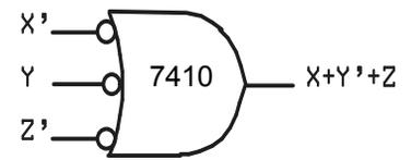
In your lab notebook, include the SOP equation for F and its corresponding circuit diagram from Exp 6.2 as well as the circuit diagram created here. Remember to use DeMorgan gate symbols but only where they are needed. If you use only normal symbols throughout, it will not be possible to follow circuit logic simply by looking at the diagram.
