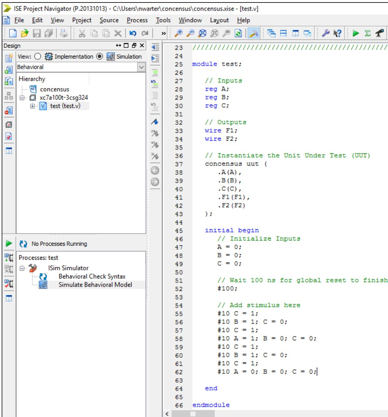
Save the file and make sure that there are no syntax errors. Make sure that your Design window still has the Simulation View clicked. Next, click on test.v in the hierarchy and then click on **Simulate Behavioral Model** under the **ISim Simulator** drop down in the **Processes** window.
