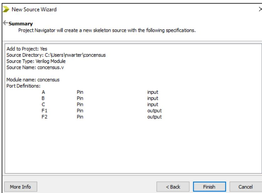
A template for your Verilog design should appear. Since we are simulating the circuit, click on the **Simulation** radial button under **Design** next to **View**. If the Verilog code is not showing in the large window, select the Verilog file (concensus.v) in the **Hierarchy** window.
