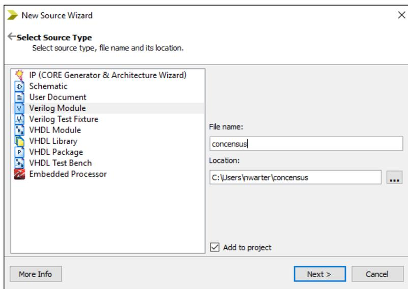
Click **Next**. Specify the names of the input and output ports. In our example, A, B, and C are inputs and F1 and F2 are outputs. Make sure to change the **Direction** of F1 and F2 to **output**.
