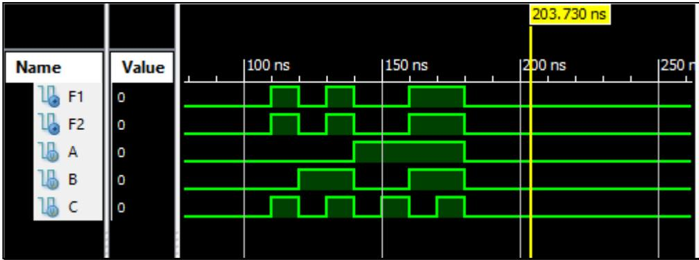
In the waveform, note that the starting at 100 ns, the values of ABC count from 000 to 111 and at 180 ns go back to 000. Reading the simulation waveform is similar to reading the oscilloscope waveforms except in this case we can see all inputs and outputs together. This is a very useful function and in fact, there are logical analyzers that are similar to oscilloscopes that capture and display multiple inputs and outputs in a digital hardware design.
