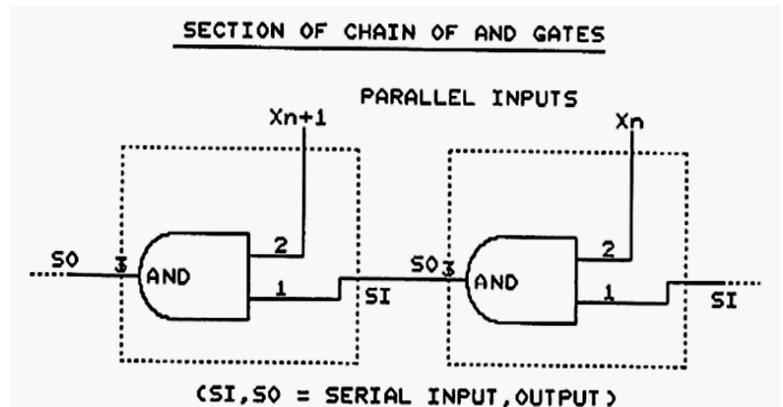
One possible application for a such a chain of AND gates would be an "All-High" detector. The output of the chain would go high only when all parallel inputs are high. (The serial input to the first gate must always be high; i.e. 5V). This really amounts to single large AND distributed along a chain.
