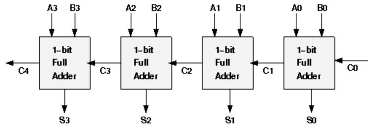
Once designed, one has only to string together as many stages as desired; i.e. a 4-bit adder would require 4 identical full-adder stages--that's the whole design. Contrast this with designing the entire 4-bit adder at once. It would take a truth-table with 9 input columns ( $A_3..A_0$ ,  $B_3..B_0$ , and  $C_0$ ), 5 output columns ( $S_3..S_0$  and  $C_4$ ), and  $2^9 = 512$  rows!
