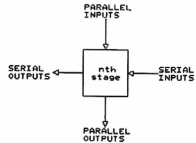
Consider, for example, an N-bit iterative adder consisting of N identical full-adder stages. Each stage includes parallel inputs  $A_n$ ,  $B_n$ , and an output sum bit,  $S_n$ . There are also serial input and output carries,  $C_n$  and  $C_{n+1}$ , which carry information from stage to stage.
