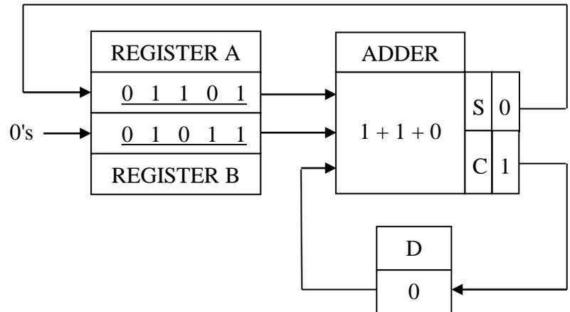
**1st clock)** When the clock is triggered, the  $S = 0$  from the previous state is brought around and shifted into the left-hand bit of register A, and the  $C = 1$  from the previous diagram is stored into D, replacing the 0 that was there.
