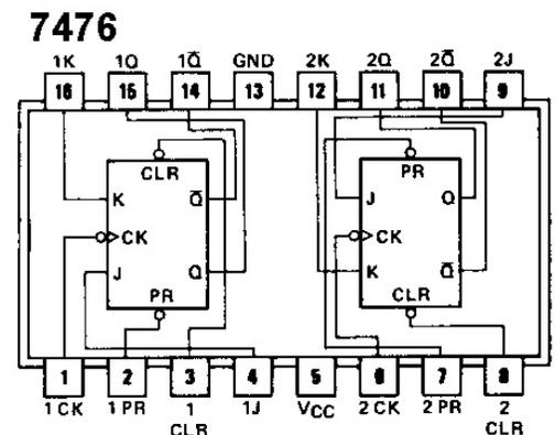
Referring to the 7476 pin assignments above, draw a wiring diagram to test the behavior of a JK flip-flop.
