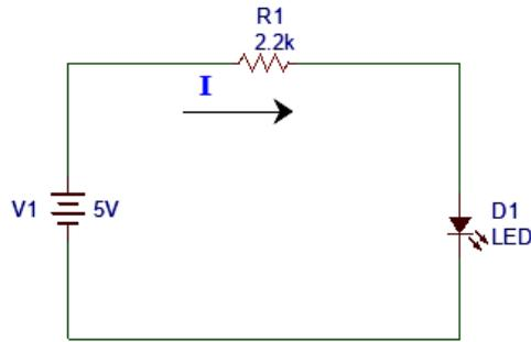
Figure 1.2. Simple electric circuit with resistor and LED.
