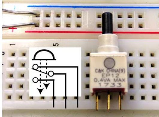
Figure 1.5. The pushbutton switch to be used in the circuit of Fig. 1-6.
