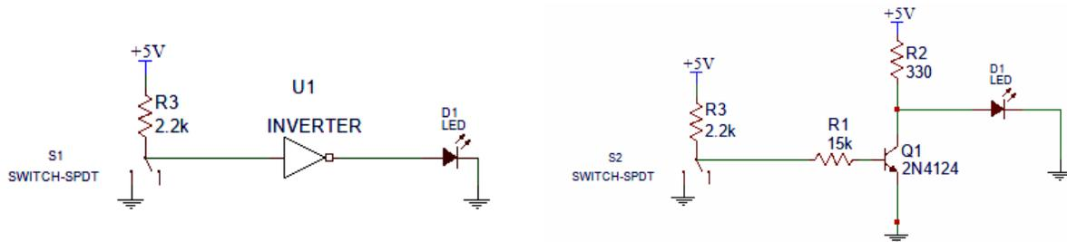
(a) Circuit built with an INVERTER gate.
