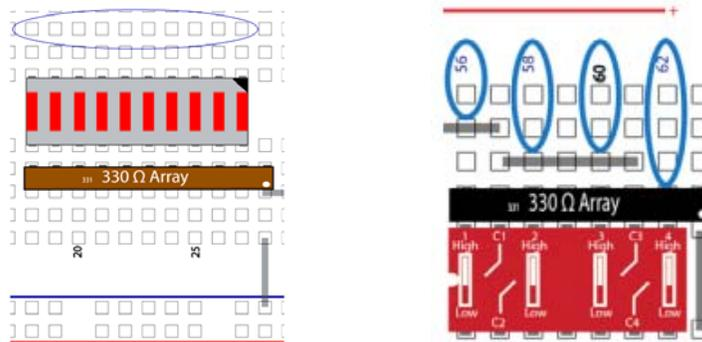
Figure 1.9. LED bargraph at left; toggle switch access diagram at right.
