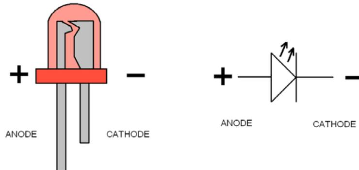
Figure 1.3. LED terminals. The anode (+) terminal has the longer lead and the cathode (-) terminal has the shorter lead.
