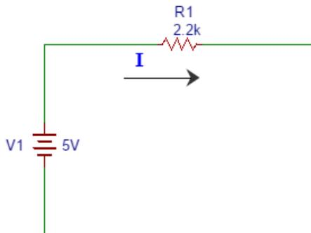
Figure 1.1. Simple electric circuit with power supply (V1) and resistor (R1)
