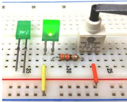
Figure 1.6. Simple resistor-LED circuit with a pushbutton switch to turn on and off the LED.
