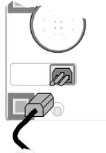
The HP 54645A/D power supply automatically adjusts for input line voltages in the range 100 to 240 VAC. Therefore, you do not need to adjust the input line voltage setting. The line cord provided is matched by HP to the country of origin. Ensure that you have the correct line cord. See table 1-1.
